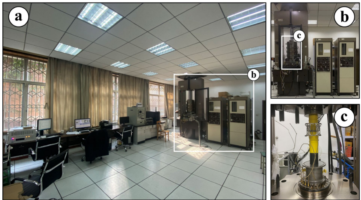
Fig. 2. Conventional triaxial compression by the MTS 815 Flex Test GT rock mechanics test system and AE monitoring system by the PCI-II.
