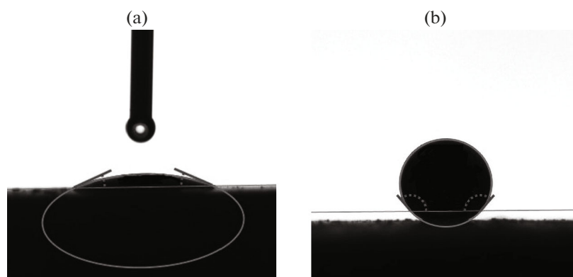
Fig. 3. Image of a water droplet on (a) the initial and (b) modified tungsten oxide powder.
