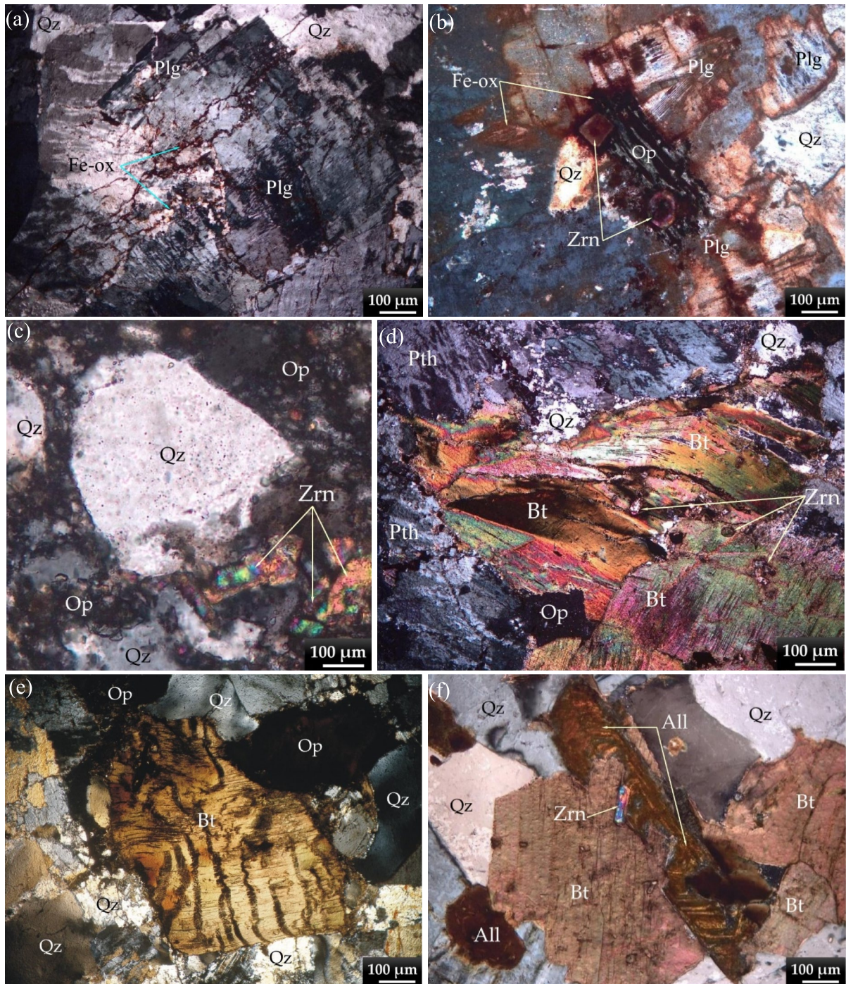
Fig. 3 Photomicrographs showing the petrographical characteristics of syenogranite at Nikeiba, SED of Egypt. a Cracked crystals of antiperthite filled with iron oxides; b Plagioclase stained with iron oxides, and associated with zircon; c Zircon enclosed in quartz and stained with iron oxides; d Twisting of
