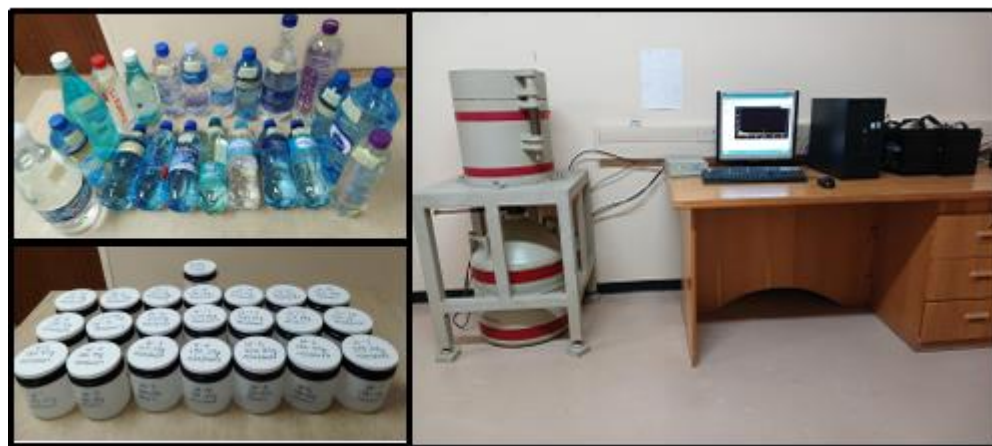
Figure 1. The experimental setup shows pictures of the collected and prepared samples as well as the HPGe gamma spectrometer for the natural spring mineral bottled drinking water analysis.
