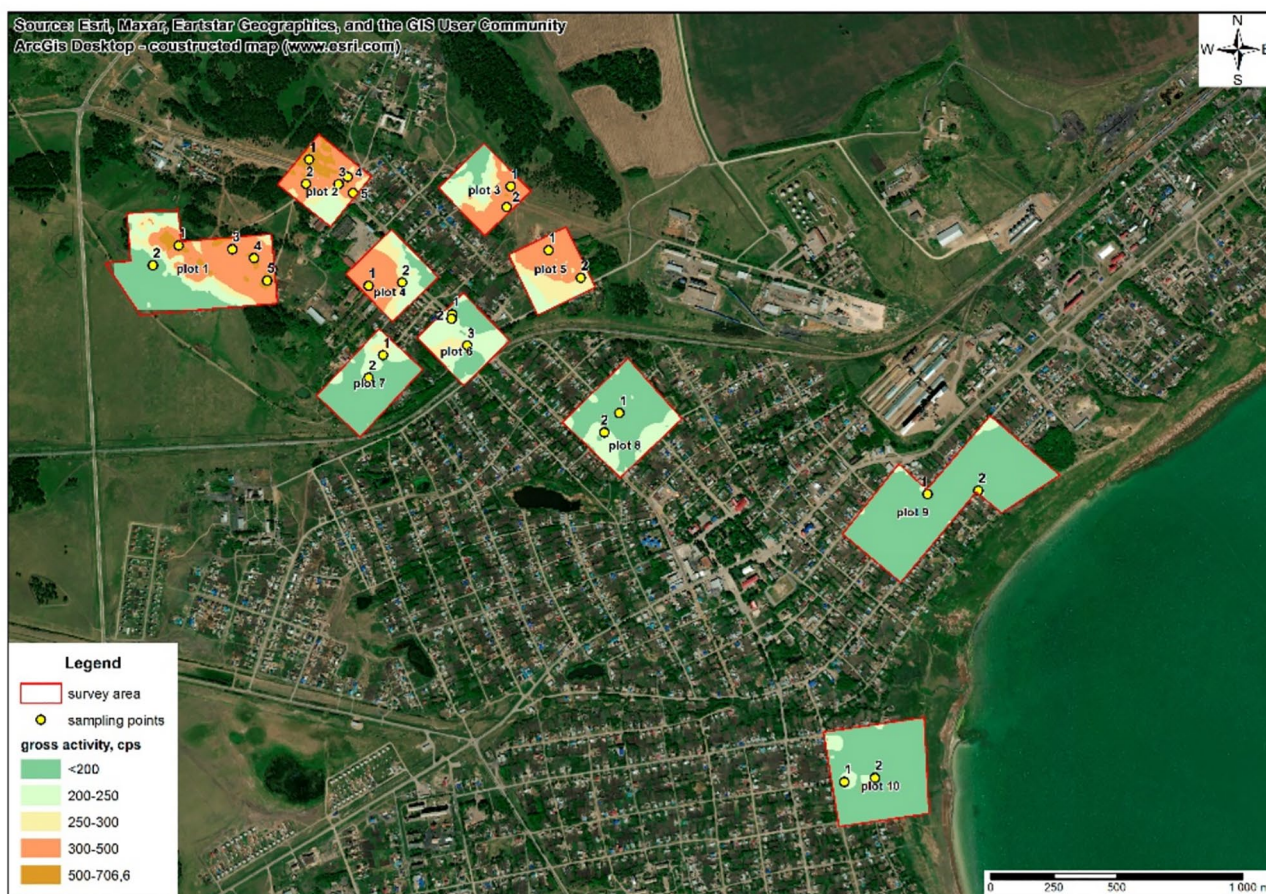
Fig. 4. Results of the pedestrian gamma spectrometry survey at 10 sites in Saumalkol village.
