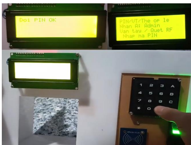
Figure 10. Experimental Run of the Smart Door Lock System Model.
