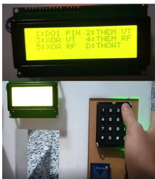
Figure 11. Experimental Run of the Model with Password Setting Function Using the Key Matrix.
