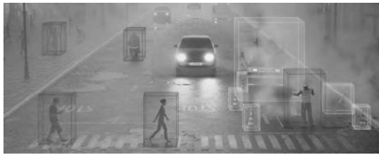
Figure 1. Sensor fusion intelligently processes raw data from different sensing devices to determine vehicle surroundings like lane markings, pedestrians, cyclists, vehicles, and street signs
