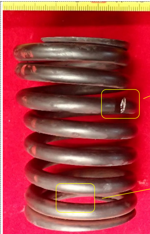
Figure 1. Macroscopic appearance of the fractured spring.
