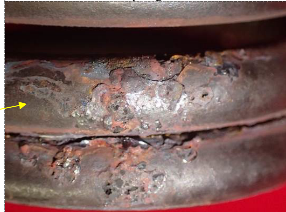
Figure 3. The localized surface of the fractured spring.
