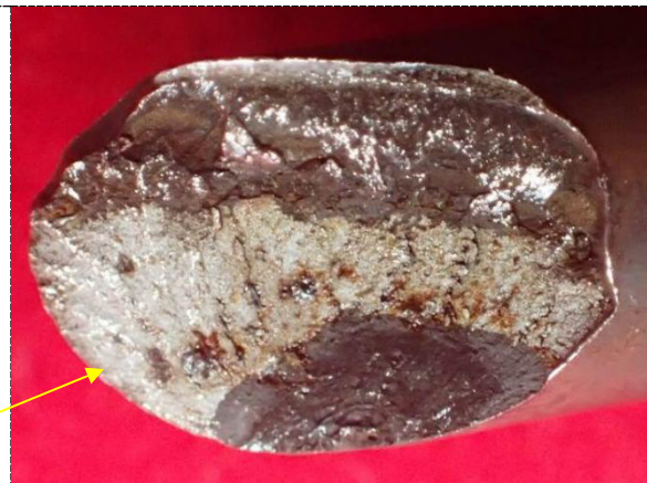
Figure 2. The fracture failure surface of the spring.
